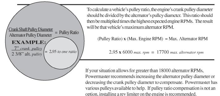
Excessive RPMs can cause the alternator fan to flex and contact the drive belt. This could cause property damage and/or personal injury. In addition to RPMs, there are other factors that will substantially increase the likelihood of alternator fan-to-belt contact.
