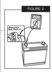
post (+) and the ground post (-). Voltage should be 13.8~14.5VDC. Readings above 15.5VDC indicate a defective alternator and readings below 12.7VDC indicate that the alternator is not functioning or cannot supply the current amperage needs of the vehicle at this engine speed.
